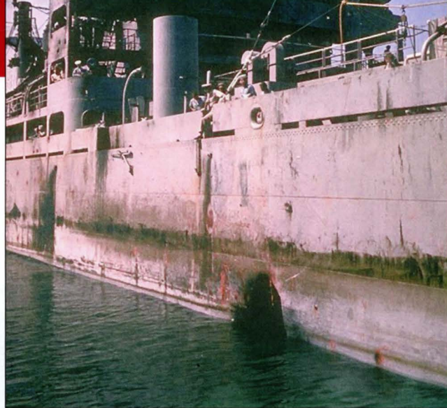
The torpedo hit Liberty at and below the waterline, creating a 24- by 39-foot hole in her hull.
